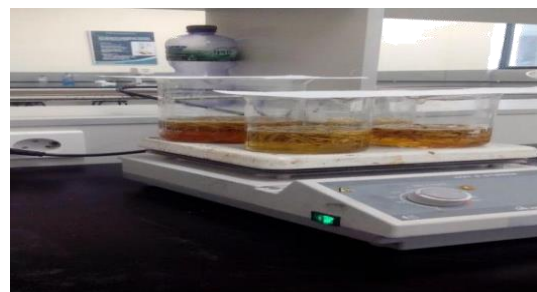
Fig 8: Alkaline treatment of sugarcane bagasse at 60 °C
