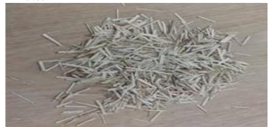
Fig 7: Sugarcane Bagasse After Washed with Pressurized Water and Dried.
