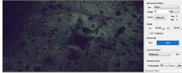
Fig 17: Hardness value image of Polyester bagasse
