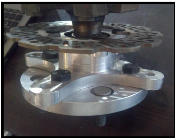
Fig. 6 Actual assemblies of Knuckle and Hub
