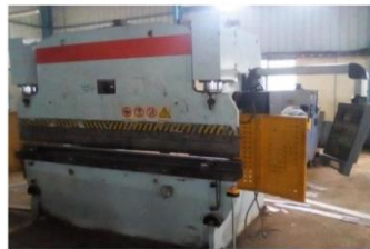
Figure 2: Hydraulic press bending machine
