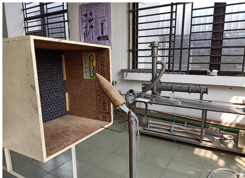
Figure 4: Experimental setup of the projectile for measuring static pressure.
