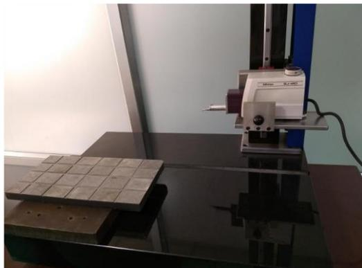
**Fig. 7: Surface Roughness Measuring Setup**
