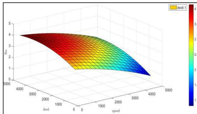
**Fig. 10: Effect of Feed and Speed on Ra**
