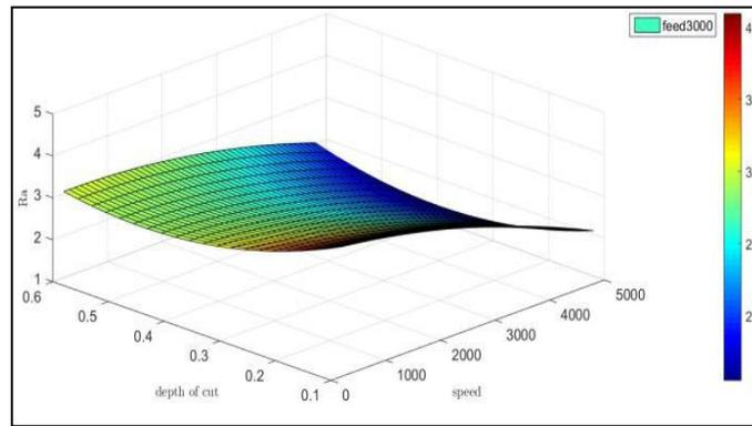
**Fig. 9: Effect of Speed and Depth of Cut on Ra**
