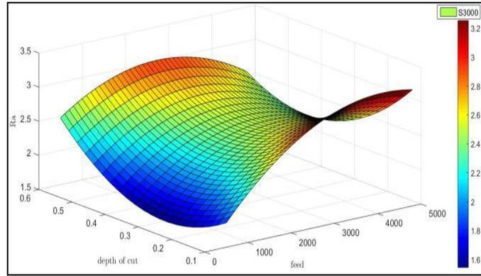
**Fig. 8: Effect of Feed and Depth of Cut on Ra**
