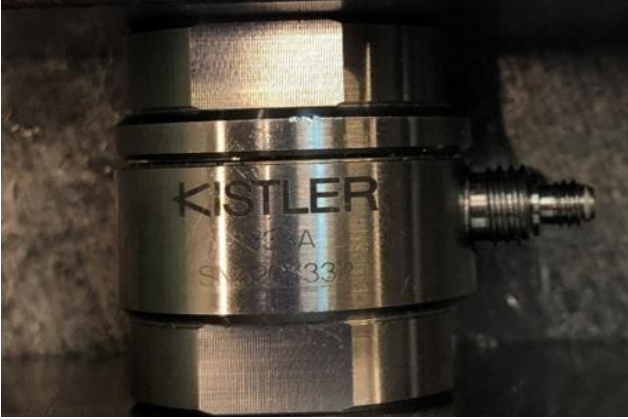
Fig. 2: Force measurement sensor used in experiments
