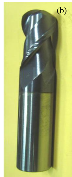
Figure 1. (a) Close up view of Experimental setup (b) Ball end mill tool and (c) Machined workpiece
