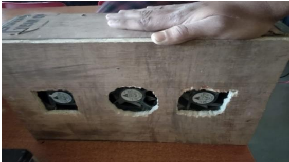
Fig:6 Exhaust fans arrangement in Peltier cooler
