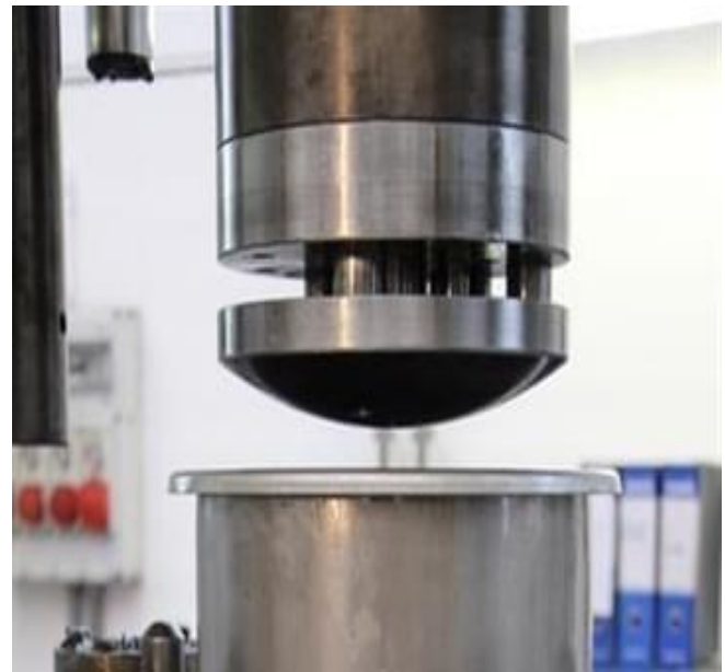
Figure 1.4 Deep drawing process
