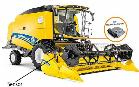
Fig 5. How to place the sensor and ECU on the combine
