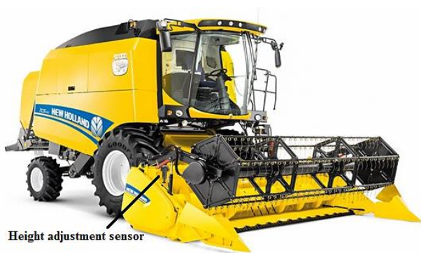
Fig 4. How to place the height adjustment sensor on the combine
