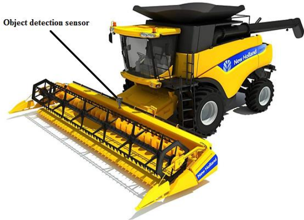
Fig 1. How to place the object detection sensor on the combine
