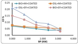
The CO emission increases with increase in load. Blends of biodiesel give less CO emission than diesel. The oxygen content in the biodiesel would have
