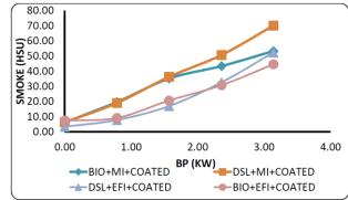
The heterogeneous combustion mixture in CI engine results in different air fuel ratio at different places inside the combustion chamber. The rich mixture is formed in the region near the nozzle and in the inner core of the droplet. Due to high temperature in absence of oxygen the fuel undergoes pyrolysis to form smoke. The
