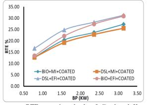
BTE at various loads of diesel and Karanja oil methyl ester blends. The increase in density of the blends increases the mass of the fuel injected inside the cylinder which results in increased time for evaporation of the fuel droplet. With increase in engine power output there is a rise in BTE for all the fuels. It is seen that K20D80 resulted in BTE in similar fashion as Diesel operation at all operating conditions. The BTE of EFI with Diesel is slightly higher than the MI with
