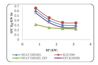
load. The reason is high cylinder temperature & better fuel combustions of fuel for K20D80 SFC is lower due to low calorific value.
