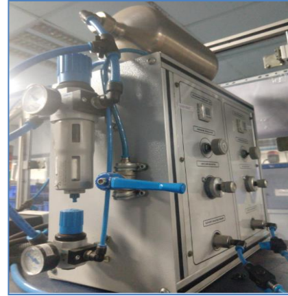
Fig 9: Crack-off test operating panel
