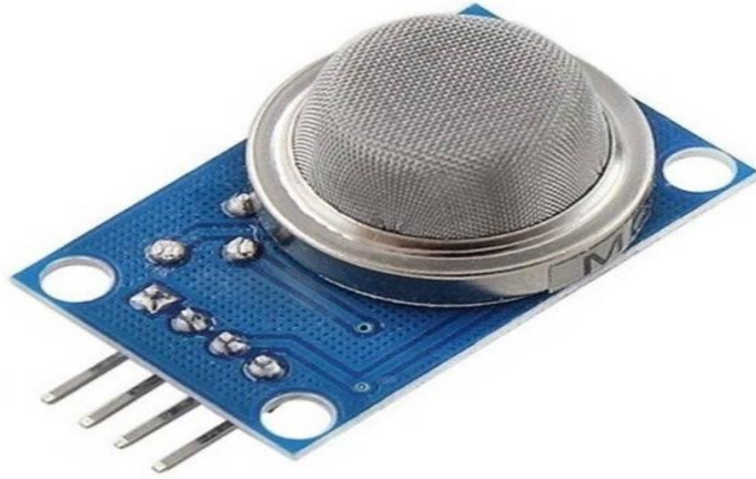
Fig 2. Gas detection sensor
