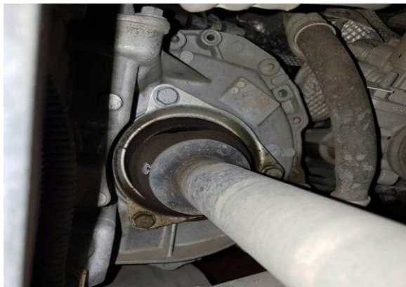
Fig 2. Rupture of the axle shaft duster
