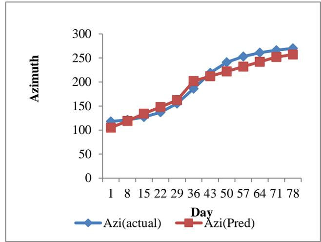
Fig. 3 Azimuth (actual) against azimuth (predictive) for day 1-78 at 7:00 -18:30
