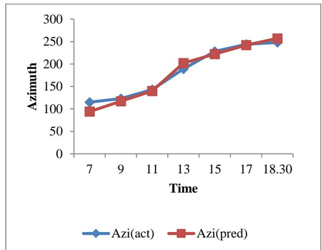
Fig. 4 Azimuth (actual) against azimuth (predictive) for day 1 at 7:00 -18:30
