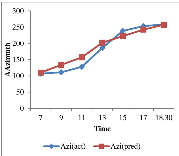
Fig. 5 Azimuth (actual) against azimuth (predictive) for day 45 at 7:00 - 18:30
