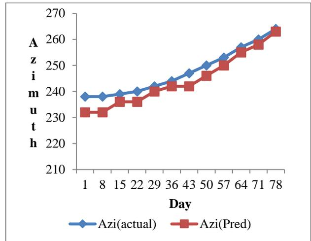
**Fig. 1 Azimuth(actual) against azimuth (predictive) for day 1-78 at 16:00**
