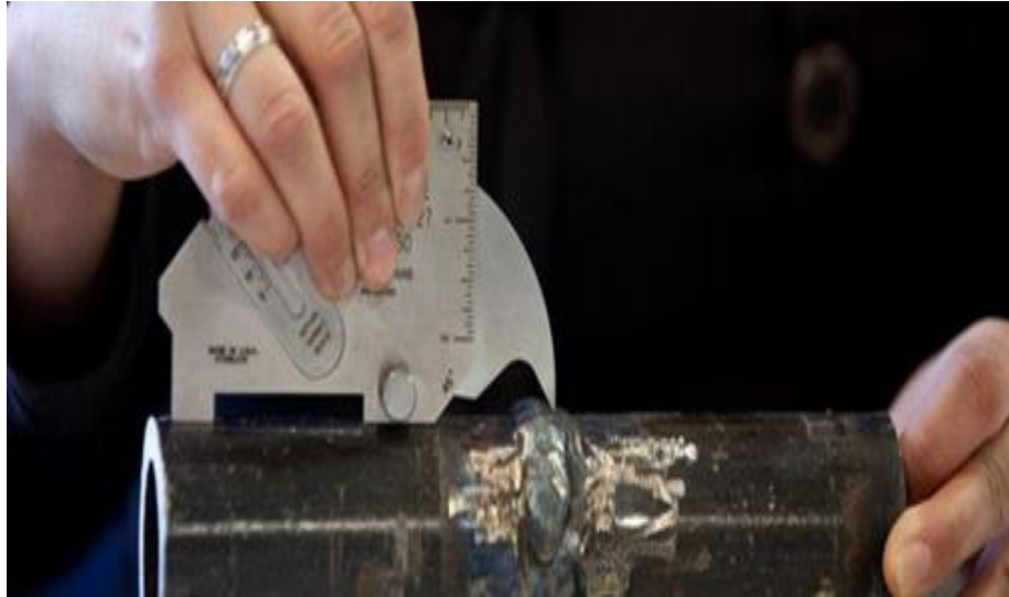
Fig. 1 Visual inspection for TIG welding
