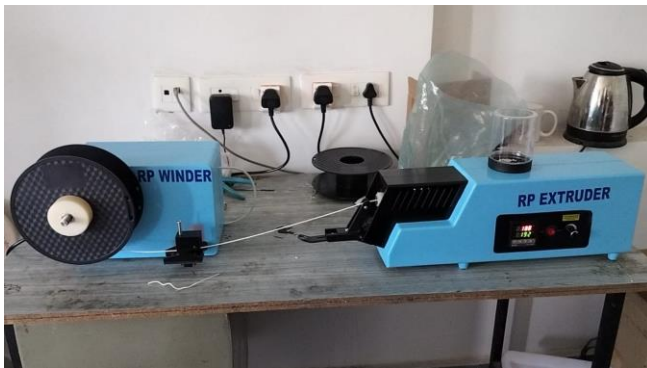
Fig. 2 Composite filament making process
