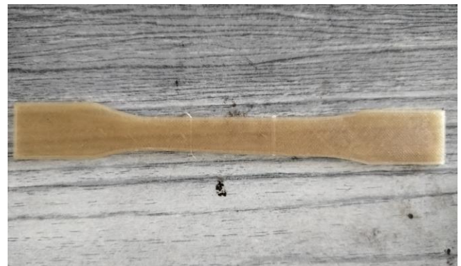
Fig. 4 3D printed tensile test specimen
