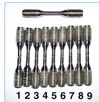
Fig. 3 Un-notched (top) and notched (1-9 below) fatigue specimens
