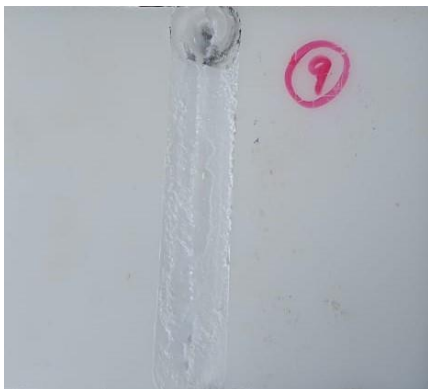
Fig. 6 Friction stir welded specimen
