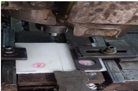
Fig. 4 Workpiece arrangement on milling machine
