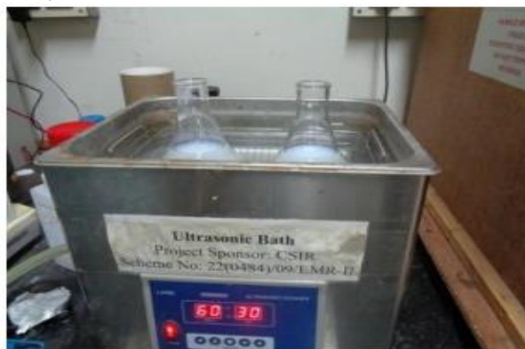
Fig. 3(a) Preparation of biodiesel-nanoparticle mixing process through Ultrasonicator
