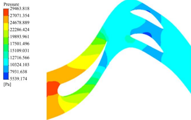
Fig. 7 Contours of static pressure at the last stage of the steam turbine in a 2D study
