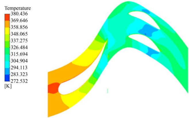
Fig. 9 Contours of temperature at the last stage of the steam turbine in a 2D study
