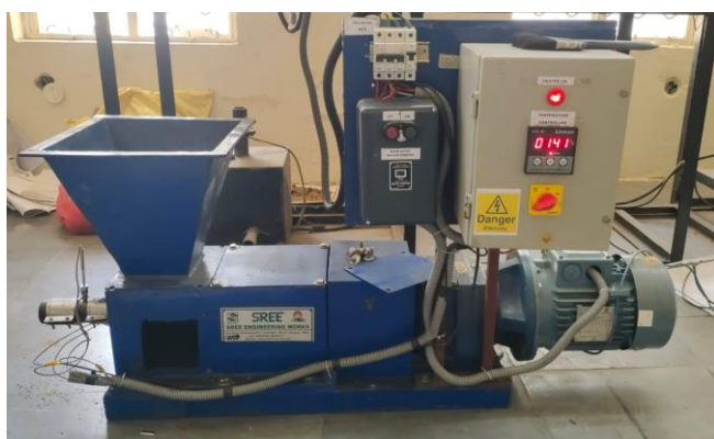
Fig. 6 Fabricated screw briquette machine
