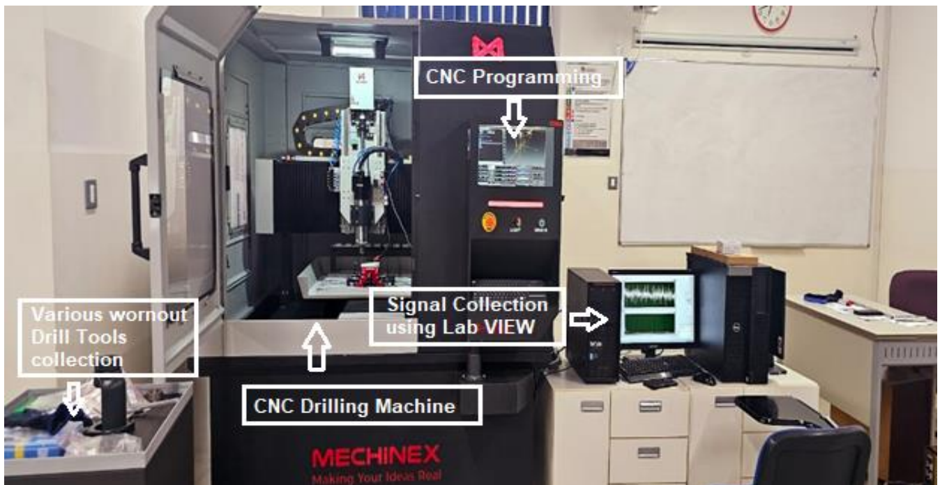
Fig. 2 Signal collection from the CNC drilling machine
