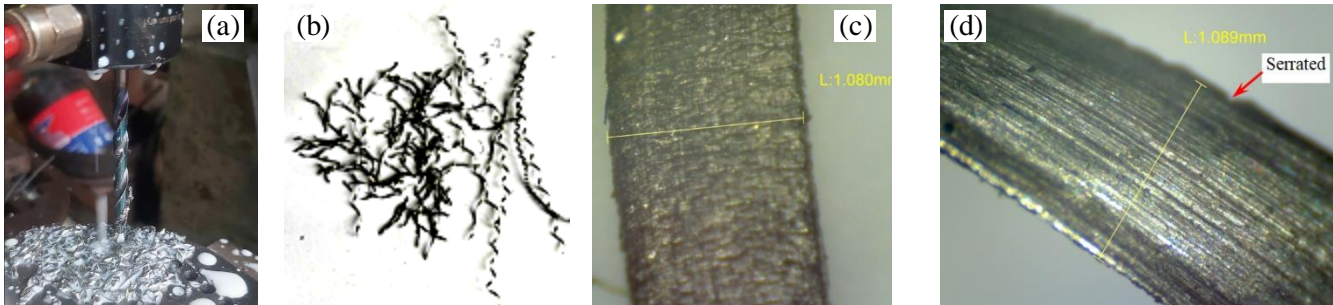
Fig. 4 (a) Drill bit after retraction, (b) Chip morphology, (c) chip free surface, and (d) Chip contact surface, observed when drilling under nanofluid lubrication.
