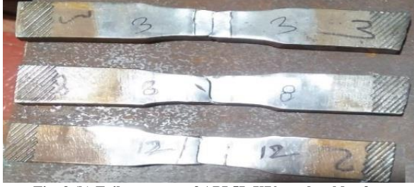
Fig. 3 (b) Failure zones of API 5L X70 steel welds after
