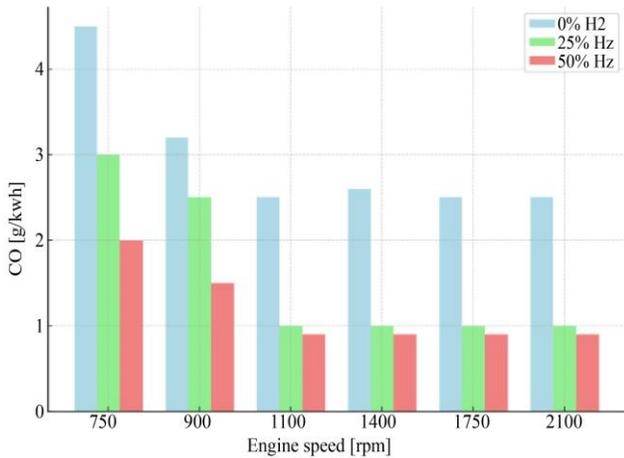
Fig. 9 Reducing CO emissions using hydrogen fuel in diesel engines.
