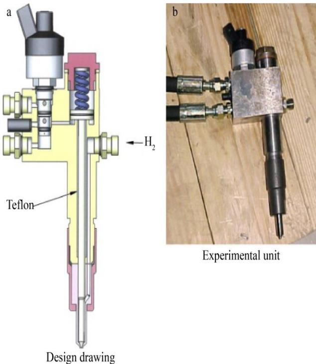
Fig. 2 Hydrogen direct injection technique [2]
