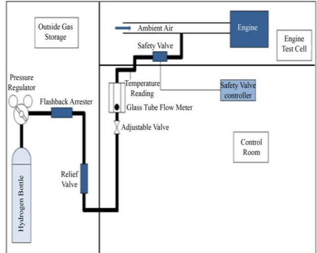
Fig. 3 Hydrogen supply into the intake manifold
