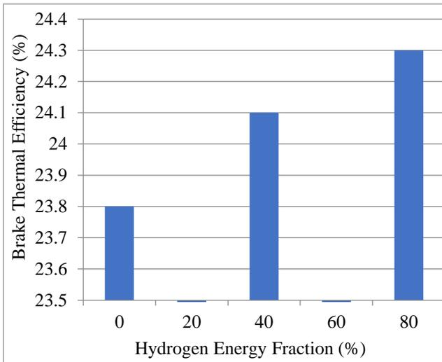
Fig. 5 Increase brake thermal efficiency with H2 increase
