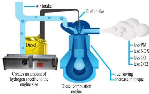
Fig. 4 Enrichment air with Hydrogen in CI engine
