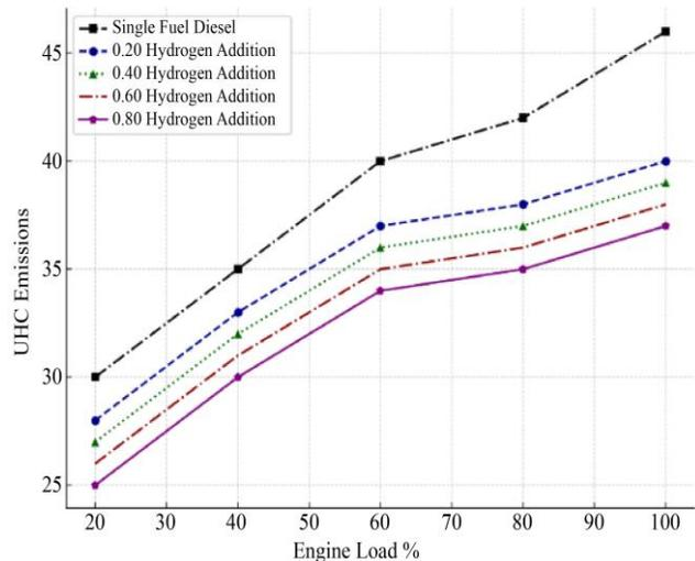
Fig. 8 Reducing HC emissions using hydrogen fuel
