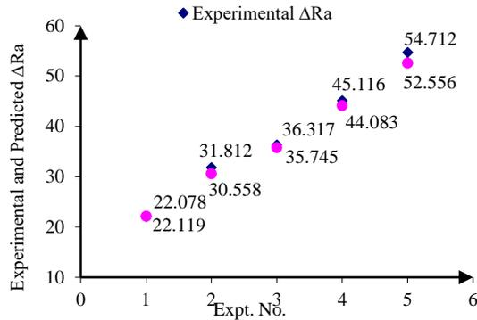
Fig. 8 Confirmatory tests, experimental vs. Predicted  $\Delta Ra$
