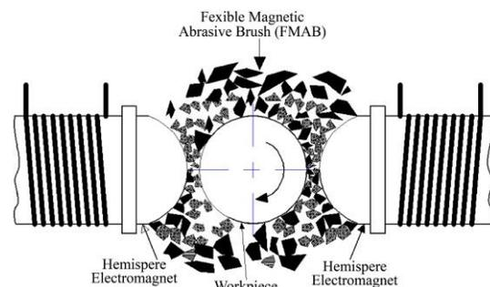
Fig. 1 Schematic of the MABF
