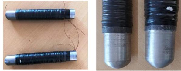
Fig. 3 Hemisphere electromagnets
