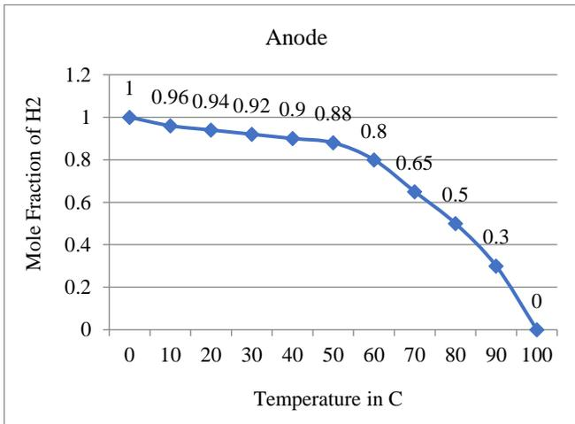
Fig. 11 Mole fraction of H2 vs Temperature of cell
