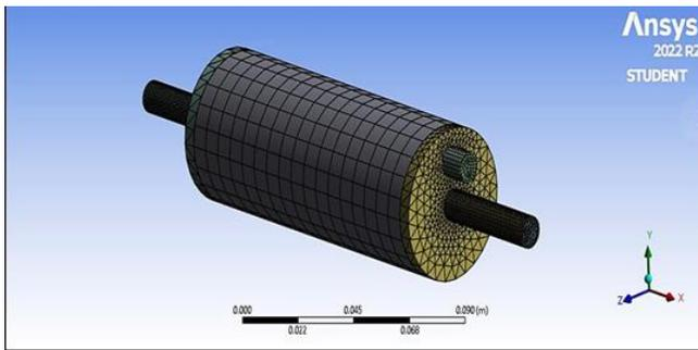
Fig. 7 Mesh Generation and Boundary Layer Refinement in the T-PEMFC Model
