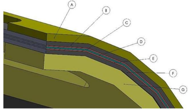
(A- Cathode, B- GDL for O<sub>2</sub>, C and E- Catalyst, D- PEM, F - GDL for H<sub>2</sub>, G- Anode)
