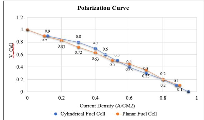
Fig. 8 Polarization curve (comparison of cylindrical and planar outputs)
