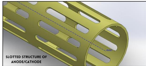
Fig. 2 Slotted structure of anode and cathode current collectors
