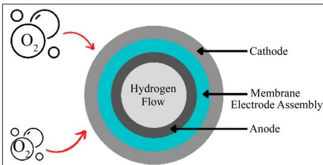
Fig. 1 Cut section view of cylinder fuel cell
