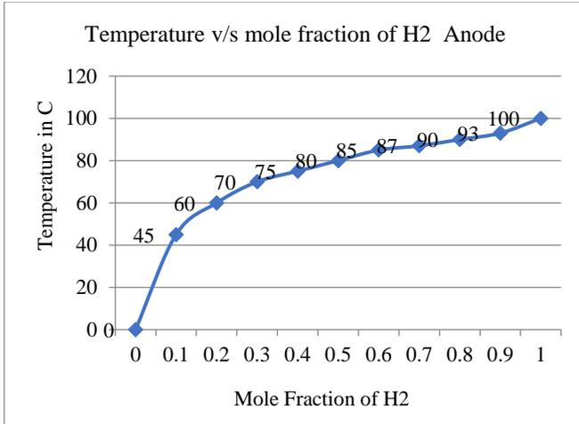
Fig. 10 Temperature of cell vs the mole fraction of H2O
