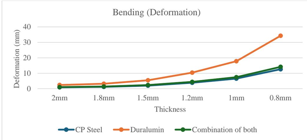
Fig. 5 Maximum deformation for pitching
