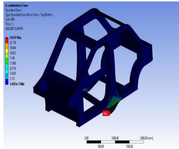
Fig. 4 Max.stress in pitching for combination of metals 2mm thick
