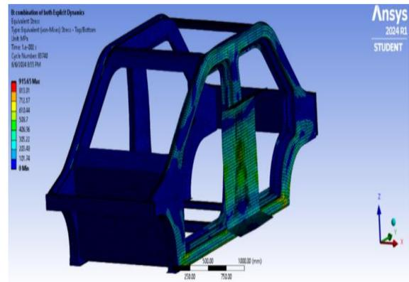
Fig. 16 Maximum stress for side crash analysis of combination material for 2 mm thickness
