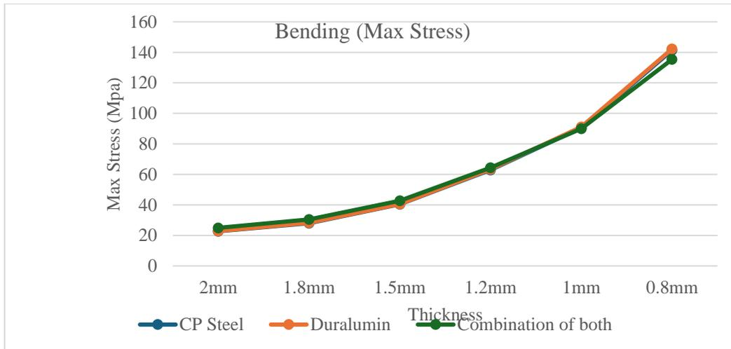
Fig. 6 Maximum stress for pitching
