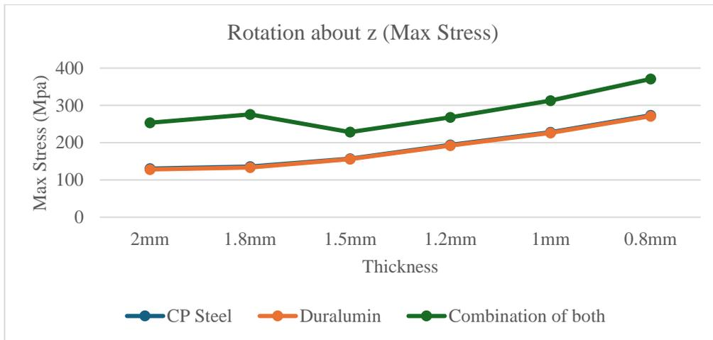
Fig. 10 Maximum stress for steering
