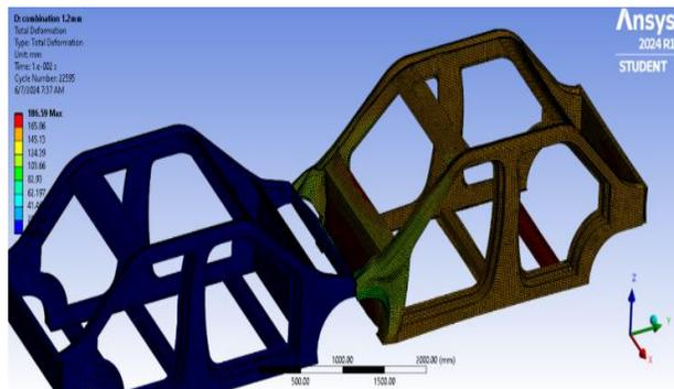
Fig. 19 Total deformation of the combination of materials in frontal impact for 1.2mm thickness
