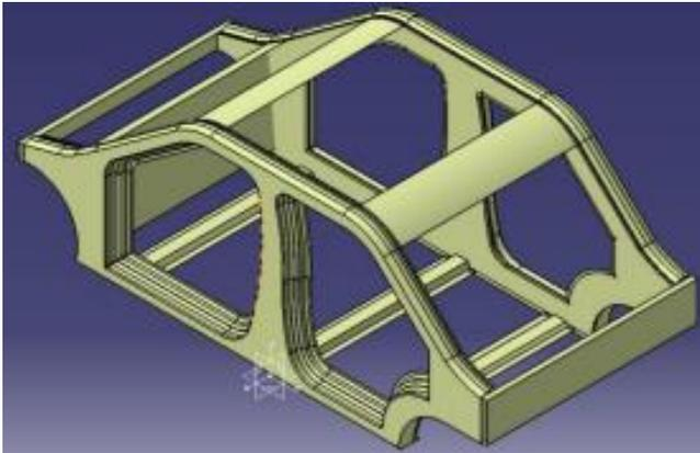
Fig. 1 Geometric model of BIW structure
