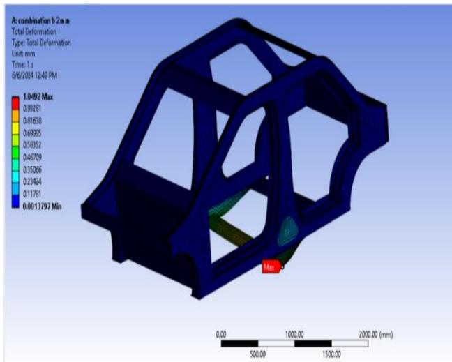
Fig. 3 Deformation in pitching for the combination of metals 2mm thick
