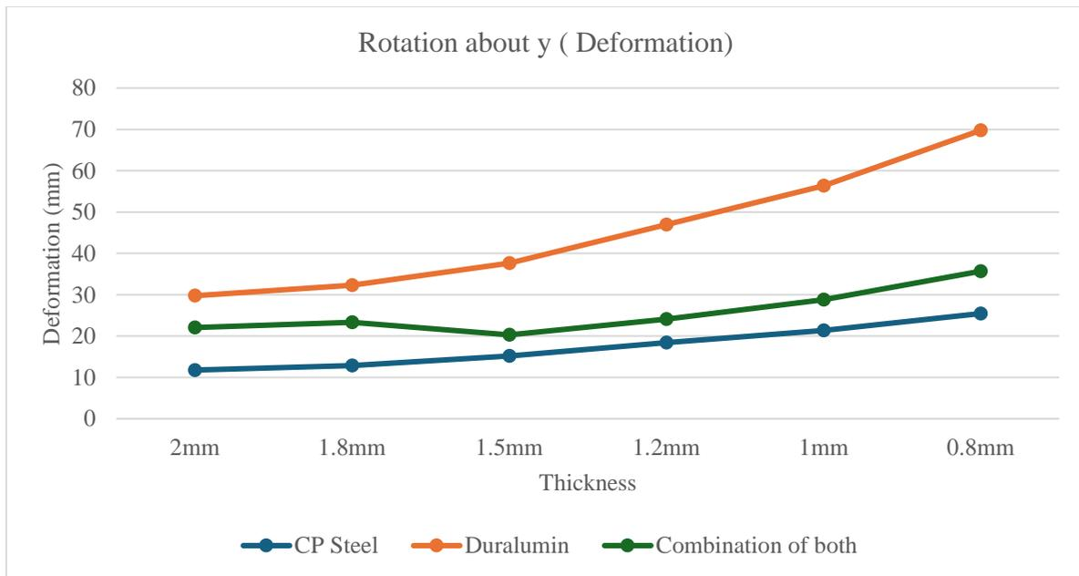
Fig. 13 Maximum deformation for pitching
