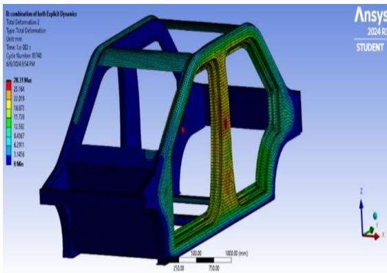
Fig. 15 Total deformation for side crash analysis of combination material for 2 mm thickness
