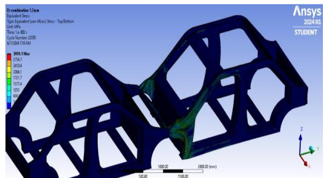
Fig. 20 Maximum stress of combination of materials in frontal impact for 1.2mm thickness
