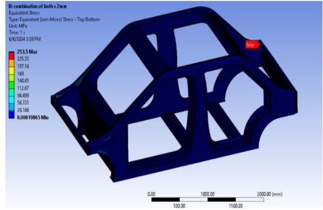
Fig. 8 Maximum stress of steering for the combination of metals 2mm
