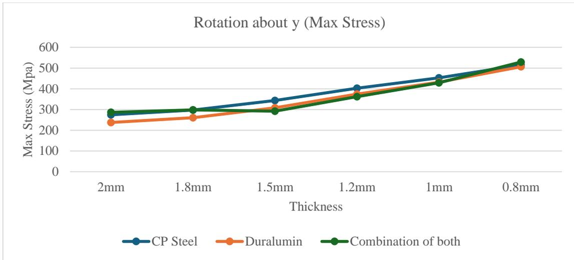
Fig. 14 Maximum stress for rolling
