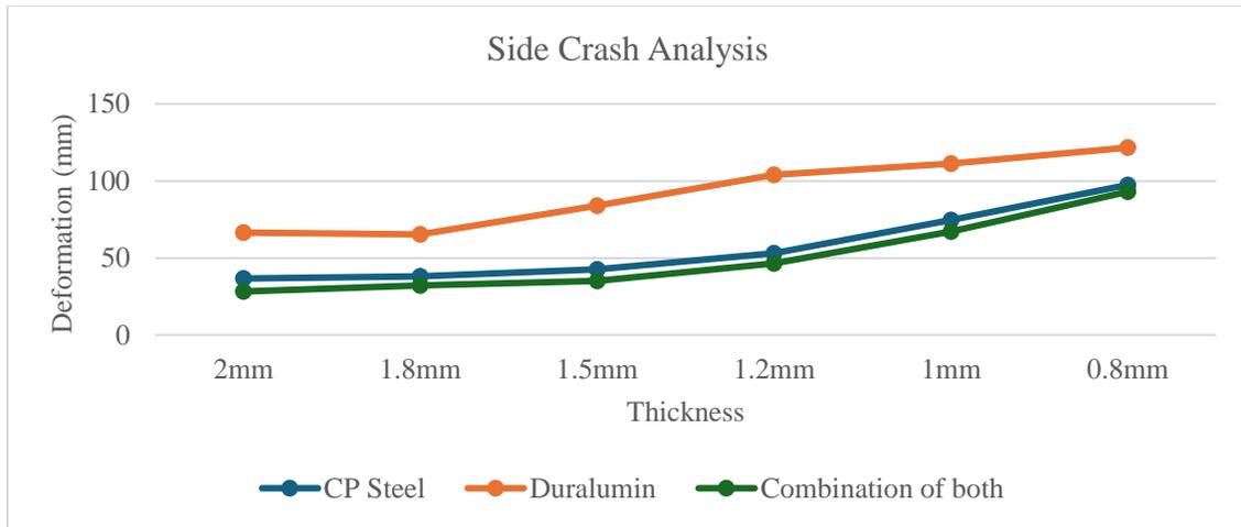
Fig. 17 Maximum deformation for side crash
