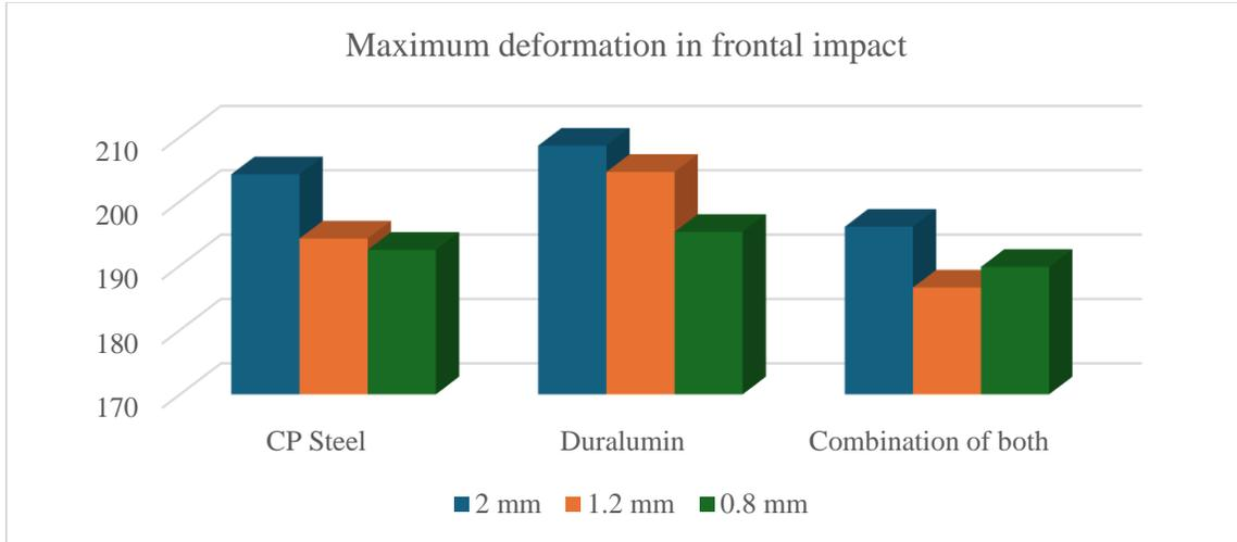
Fig. 21 Deformation in frontal impact
