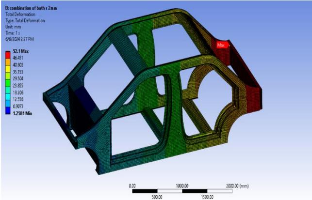
Fig. 7 Total deformation of steering for the combination of metals 2mm
