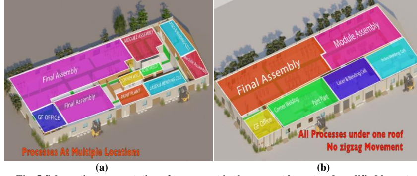
Fig. 5 Schematic representation of movement in the current layout and modified layout
