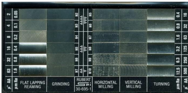
Fig. 3 Rubert surface roughness comparator
