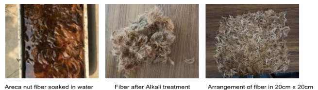
Fig. 1 Preparation of composite sheets made with areca nut husk fiber
