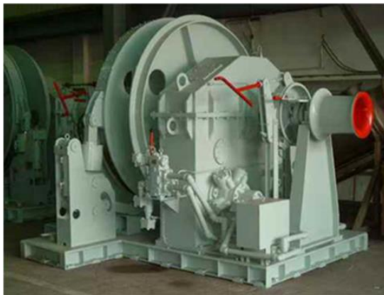
Fig. 1 Ratchet-type anti-impact reel
