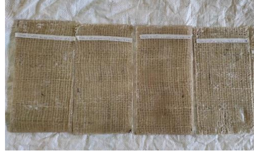
Fig. 4 Samples with varying sisal fiber and UP resin mass fractions
