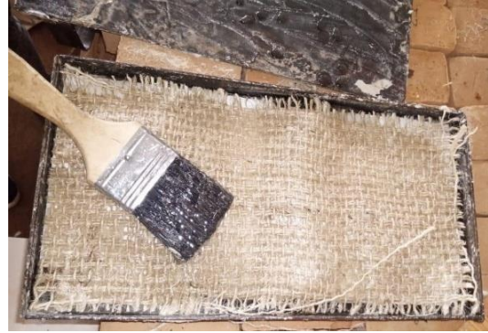
Fig. 3 Laying up of the sisal mat and impregnation with UP resin
