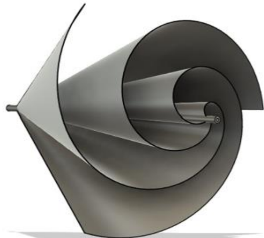
Fig. 4 Geometrical model of logarithmic wind turbine
