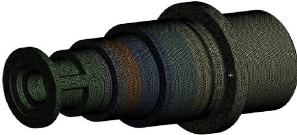
Fig. 2 Housing finite element model
