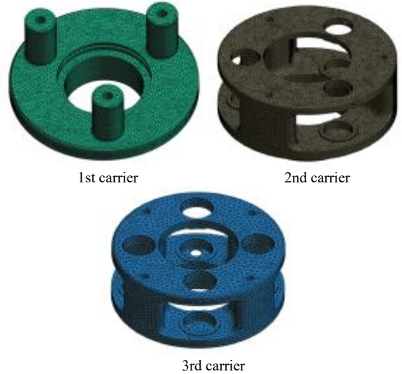
Fig. 4 Carrier finite element model
