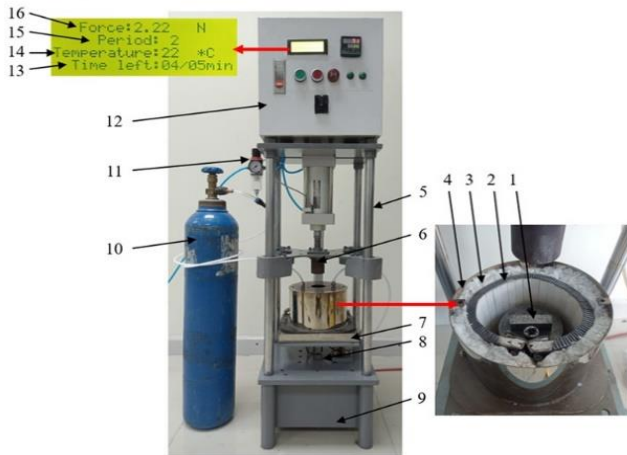
Fig. 1 Schematic of the custom nano-silver sintering system showing the heating module, pneumatic loading assembly, and sensor-control unit. The setup includes the mold and heater block, insulation stack, pneumatic regulator with load-cell feedback, and the temperature/force displays used for process monitoring. The arrangement provides controlled temperature-pressure application and stable bondline alignment during sintering
