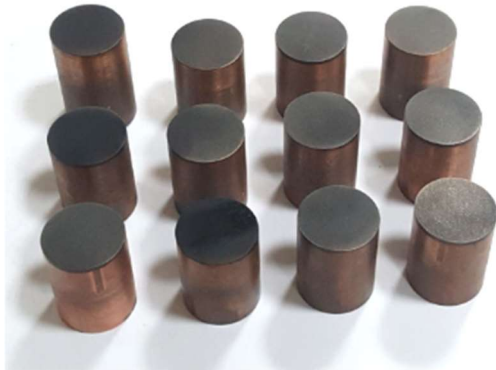
Fig. 7 Copper electrode surface after EDM process
