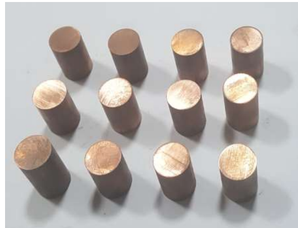
Fig. 3 Copper electrode, \text{Ø}15 \text{ mm}
