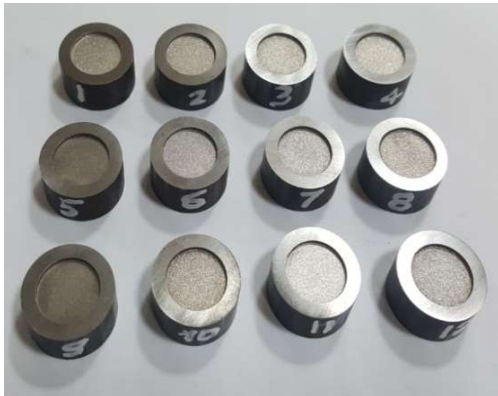
Fig. 6 9XC steel surface after EDM process
