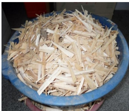
Figure 1: Wood particle (Strands)
