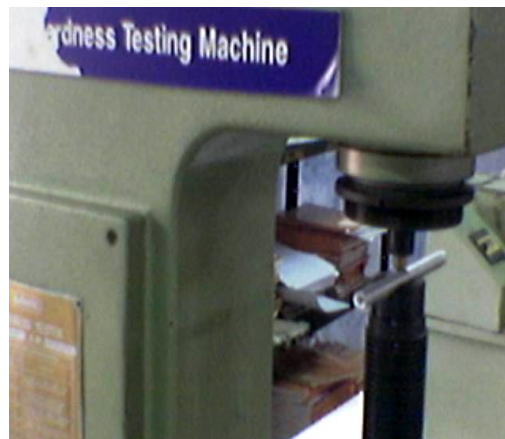
Fig. 3.2 Rockwell hardness test setup
