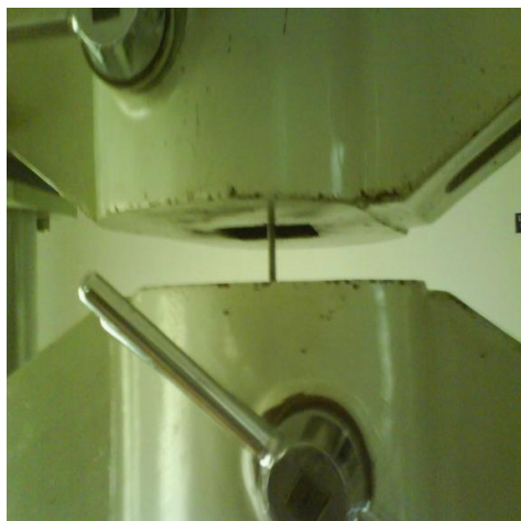
Fig. 3.1 Specimen Fixed Between the Jaws of Tensile Testing Machine
