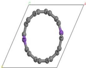
**Fig 03 (a) Ring structural diagram of 1D K doped carbon nanotube.**
