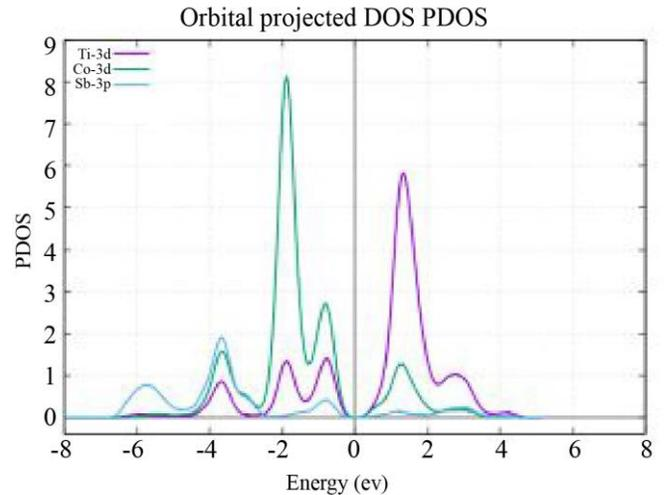
Fig. 3 Projected density of state
