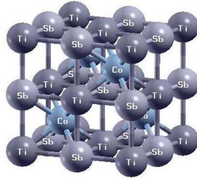
Fig. 1 Crystal structure of TiCoSb
