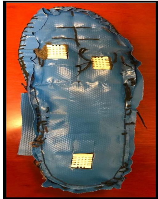
Figure 3 Diabetic Insole for monitoring temperature, humidity, and pressure.
