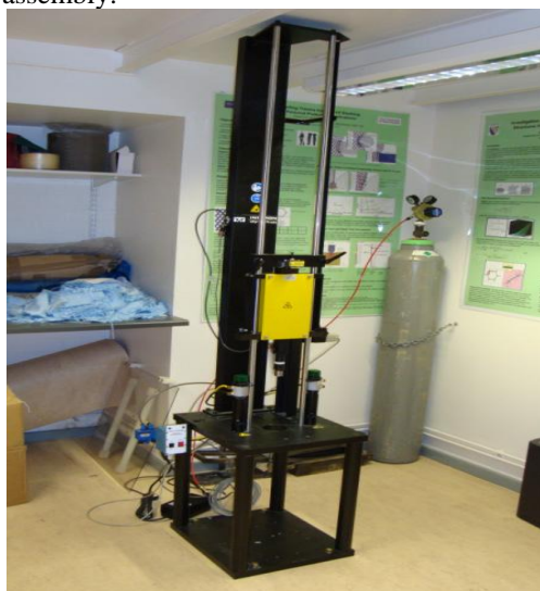
Figure 3. Dynatup 8200 Drop Weight Impact Testing Instrument
