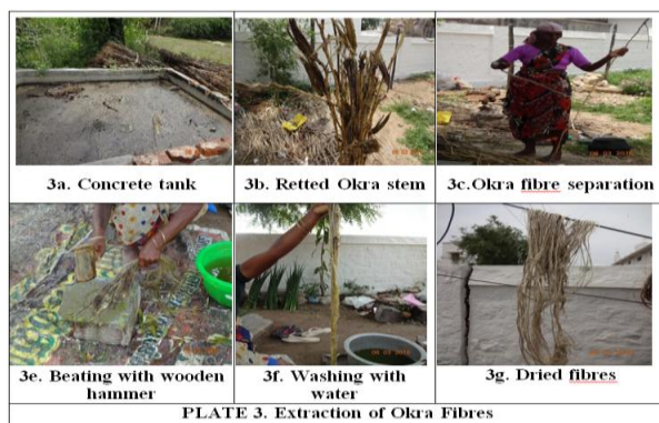
PLATE 3. Extraction of Okra Fibres
