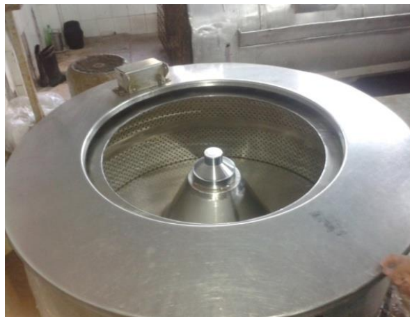
Fig: Hydro Extractor machine
