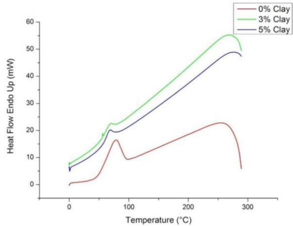
Figure 5: DSC curve of PAN Fibres
