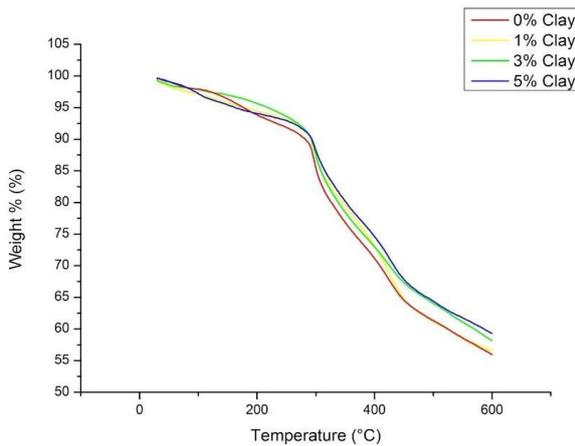
Figure 4: TGA curve of PAN Fibres
