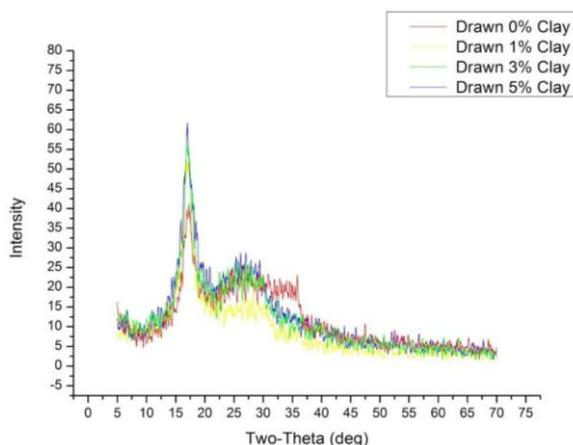
**Figure 7: XRD curves of Drawn Fibres**
