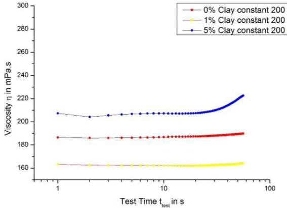
Figure 3: Viscosity-Time Characteristics of Samples
