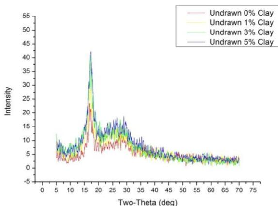
**Figure 6: XRD curves of Undrawn Fibres**
