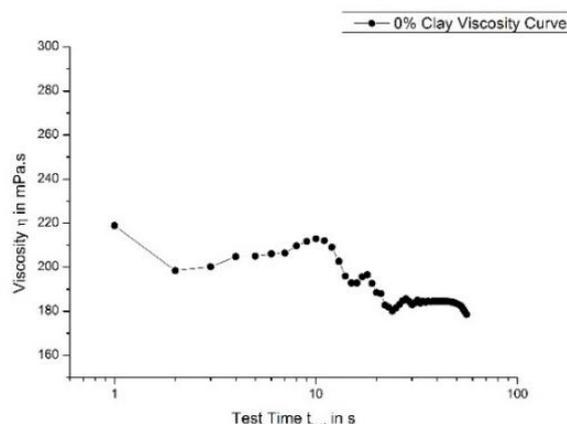
Figure 2: Viscosity curve of PAN with 0% Clay
