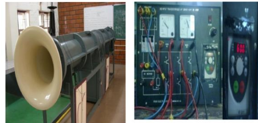
Fig 5. Ducted Axial Fan Rig & Variable frequency Drive for speed control
