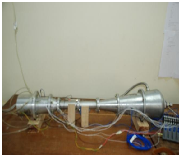
Fig.1 Experimental Setup of a Thermoacoustic Refrigerator
