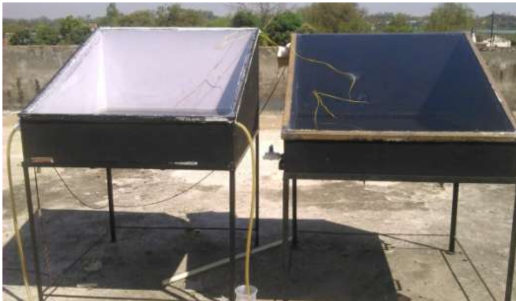
Figure1: Perspective view of conventional solar still
