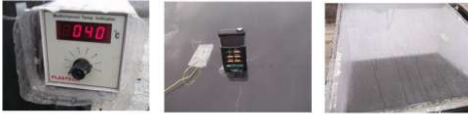
Figure3: Experimental setup of White painted (modified) and Black painted single slope solar stills
